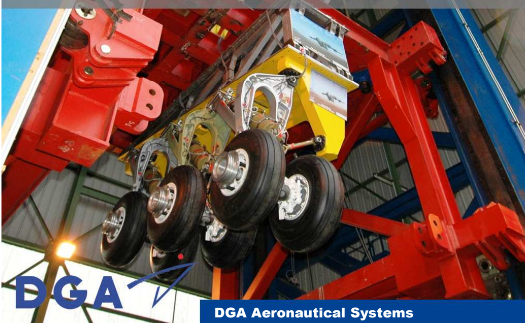
MEGA : large landing systems dynamic test
